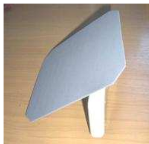
Figure 3: Si low cost substrate with dimension 156 \times 156\ \text{mm}^2
