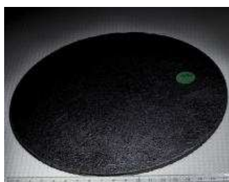
Figure 2: Spark plasma sintered Si powder based wafer, disc with d = 200 mm.
