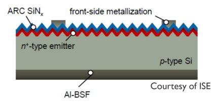
How can we further improve the industrial silicon solar cell efficiency and simultaneously reduce the cost?
