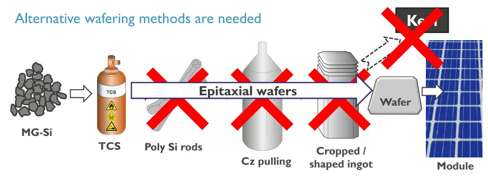
3 Direct growth of wafers from gas-phase: **Epitaxial lift-off**
