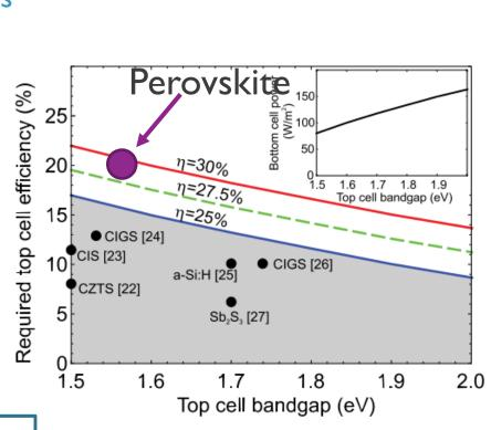
Needed: thin-film top cell with high bandgap, high efficiency, and minimal sub-bandgap absorption
